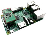
parts: (A) the transceiver hardware that is plugged on top of the RaZberry on as shown in the image above (it uses the GPIO Pins 1-10), (B) a Z-Wave controller software running on the Raspberry Pi itself. You can download a free license of Z-Way from the website razberry.z-wave.me that will work with the hardware out of the box.
